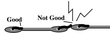
**“Solder”** When you are directed to *solder*, this means to solder the part's leads in place, and to inspect both (or all) solder connections for flaws or solder bridges. If no soldering problems are noted, nip off the excess protruding leads with a sharp pair of side cutters.
