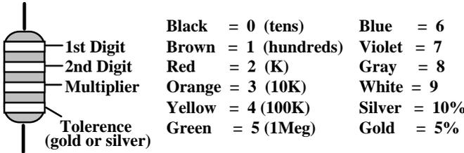
When you look at a resistor, check its multiplier code first. Any resistor with a black multiplier band falls between 10 and 99 ohms in value. Brown designates a value between 100 and 999 ohms. Red indicates a value from 1000 to 9999 ohms, which is also expressed as 1.0K to 9.9K. An orange multiplier band designates 10K to 99K, etc.
