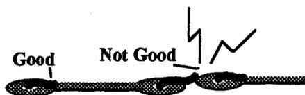
The term *solder* means to solder the part's leads in place, and to inspect both (or all) solder connections for flaws or solder bridges. Nip off excess protruding leads with a sharp pair of side cutters.
