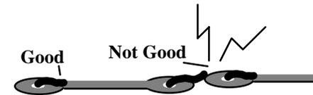
**Applying Heat:** Place the iron tip so it contacts both the component lead and pad. The objective is to heat *both* metal surfaces simultaneously. After about 1 second, apply solder to the *opposite side* of the wire from the iron tip (see below). The solder should melt due to contact with the solderable surfaces, and not from contact with the iron itself. Never melt solder on a connection by touching it to the iron tip!
