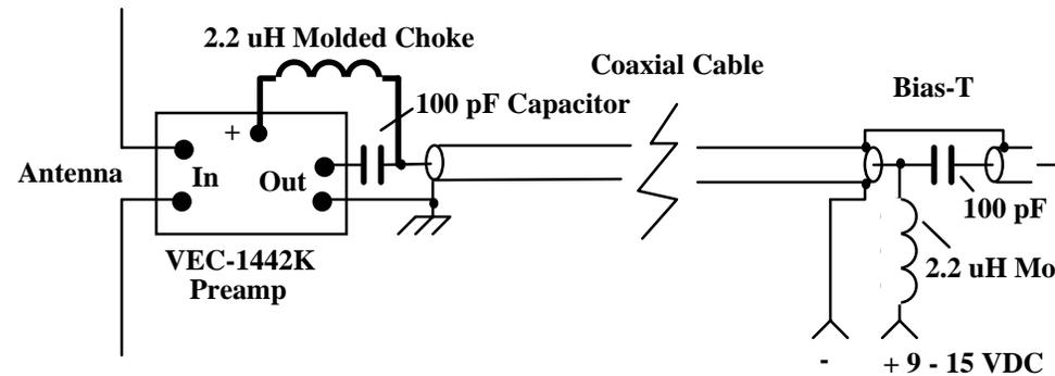
**Warning:** Never reverse-install a bias-T so DC voltage is fed into your receiver's antenna terminals. Also, never reverse-polarize the supply voltage to your preamp (swap + and - leads). In both instances, damage may result!
