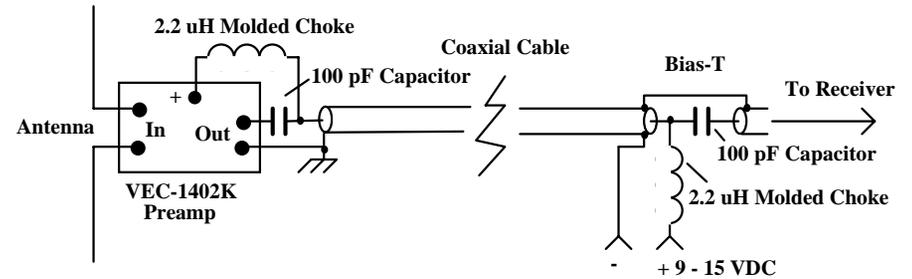
**Warning:** Never reverse-install a bias-T so DC voltage is fed into your receiver's antenna terminals. Also, never reverse-polarize the supply voltage to your preamp (swap + and - leads). In both instances, damage may result!
