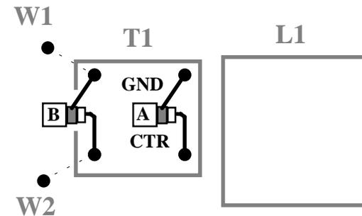
**Feeding Balanced Antennas with the Balun:**
