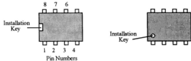
The IC body has a small notch, or *key*, molded at one end, indicating pins 1 and 8. A small dimple-like body-molding is often found adjacent to pin 1. Some IC packages may include both key indicators.
