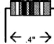
Important Note: the fourth resistor color band is for tolerance, and is not called out in the following steps.
