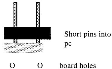
**Important Note:** When installing the two-pin jumper headers, the shorter pins are inserted into the pc board.,
