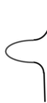
The wire insulation is removed where shown in the directions, and made into a half loop as shown above.
