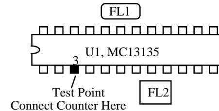
1. Connect the frequency-counter ground lead to a ground point (case or PC board).
