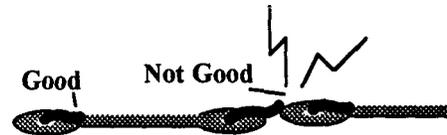
The term *solder* means to solder the part's leads in place, and to inspect both (or all) solder connections for flaws or solder bridges. Nip off excess protruding leads with a sharp pair of side cutters.
