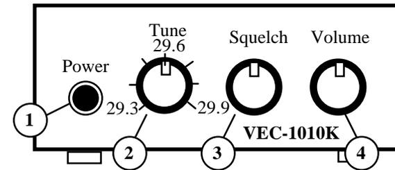
1. **POWER:** Push-on/push-off switch turns unit on and off. The VEC-1010 runs on internal battery power and shouldn't be left *ON* for extended period when not in use.
