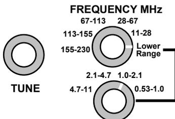
The VFO **Tune** capacitor features a reduction driver to provide smooth continuous frequency control with a small amount of overlap at each band edge.
