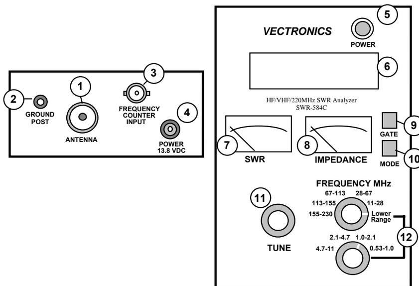
1. **Antenna Port:** SO-239 for attaching antennas and RF devices under test.
