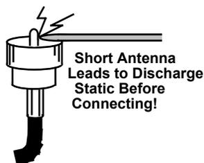
**Important Warning:** *Never applying an external voltage to the Antenna jack -- it could damage sensitive detector diodes. Also, always discharge the coax connector to bleed off static before attaching ungrounded arrays.*
