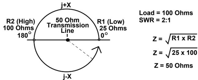
Viewed on a Smith Chart, the transformed load impedance ( $R \pm jX$ ) literally traces a circle around the characteristic impedance of the transmission line with each 360-degree rotation. The greater the mismatch, the larger the diameter of the circle. We can use this behavior in two different ways to determine the impedance of an unknown transmission line.
