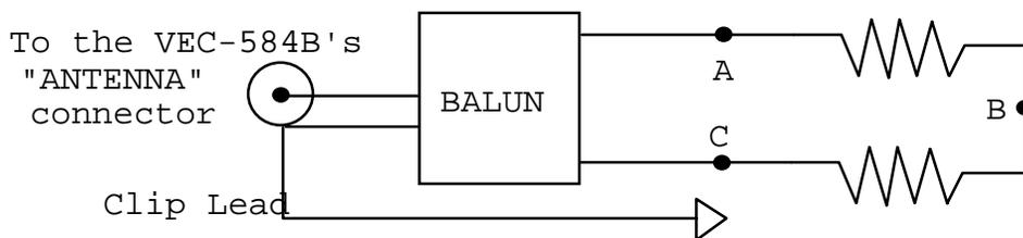
A properly designed current balun is the type most effective for maintaining current balance. It has the highest power capability and lowest loss for given materials. It should show a low SWR over the entire operating range of the balun with the clip lead in any of the three positions.
