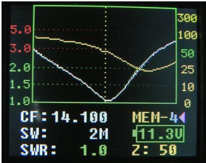
4. You can change the scan width when tune the knob and indicate purple Triangle on "SW". Push the knob for 1 second to save. FG01 will memory current CF,SW,step in next power on.
