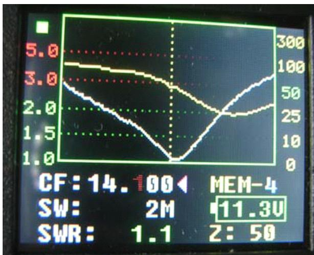
3. You can tune the knob to change the center frequency when the Green Triangle on "CF". Push the knob over 1 second can setup the step. The related number will be changed to red color, tune the knob to change the step. Light push the knob to quit, will automatic quit in 3 second.
