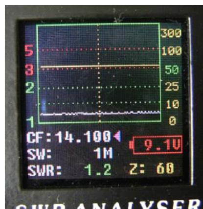
Battery indicate turns red when lower than 9.5V, must charge the battery immediately! Or will damage the battery!
