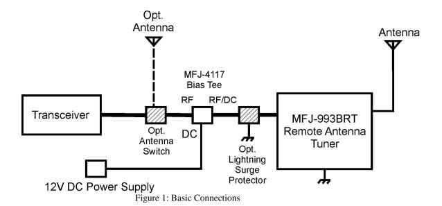
4. Connect the antenna to the tuner. Random wire or single wire line antennas should be connected to the WIRE binding post on the back of the tuner. Do not connect WIRE and coax ANTENNA at same time! Both are connected in parallel. Run the antenna connected to the wire terminal away from the tuner and not routed near the front cover to reduce the chance of RF getting into the tuner and causing it to go into bypass mode.
