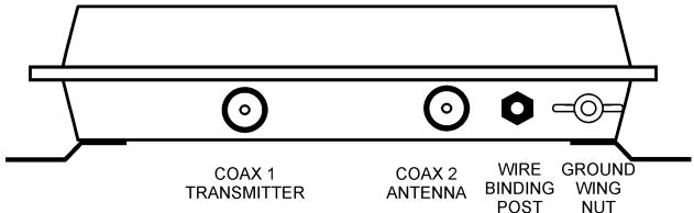
Figure 2: Side View of Connectors
