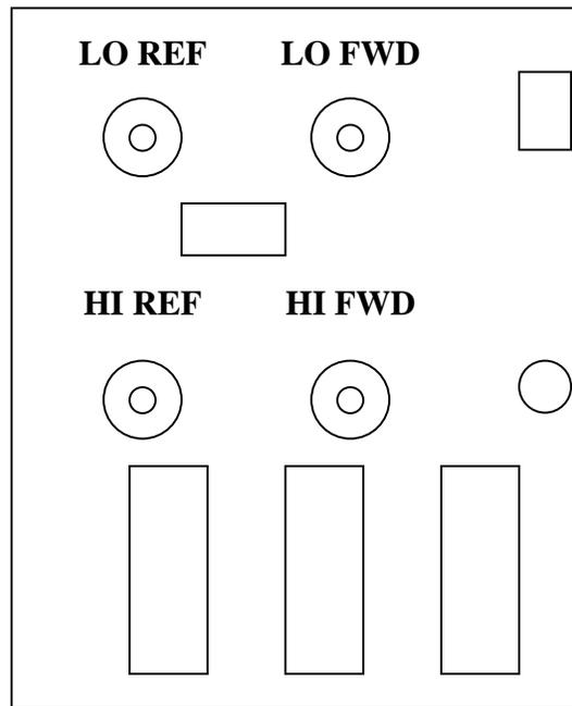
Figure 2: PCB Layout and Trim Pot Location
