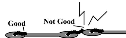
The term *solder* means to solder the part's leads in place, inspect for flaws or solder bridges, and nip off any protruding lead or pin with a sharp pair of side cutters. All solder connections will be made on the bottom (groundplane) side of the pc board.
