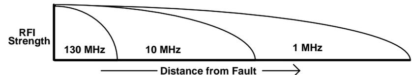
Due to standing waves, RFI varies in intensity along the powerline. This makes precise tracking at HF nearly impossible. However, near the fault, HF peaks occur progressively closer together and amplitude becomes more constant, signaling a "ballpark" location.
