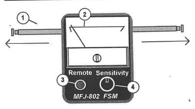
Collapsible Dipole: Balanced pickup element extend to 38" (1/2-wave on 2-meters). Adjust for resonance at VHF/UHF frequencies, or extend fully and use as a non-resonant dipole at HF. The antenna is RF-decoupled from metering circuitry, and a dipole pattern will be maintained at non-resonant frequencies.
