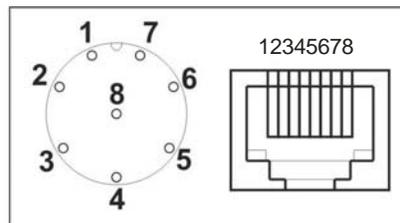
**Figure 5: Front panel view of Mic Jacks.**
