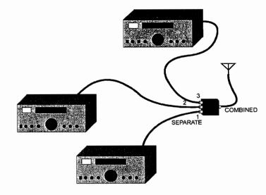
Single band radios to multi band antenna. Connect the multiband antenna to the COMBINED or MIX port and connect the proper band radios to the SEPERATE ports. . .
