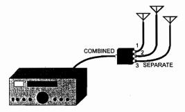
Multi-band radio to single band antennas. Connect the radio to COMBINED or MIX port and connect the correct band antennas to the SEPERATE ports.
