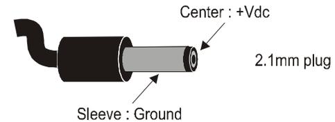
The sleeve is negative, and can be grounded or floated at the power supply. The center pin is positive, and **MUST** be ground isolated.
