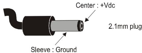
The sleeve is negative, and can be grounded or floated at the power supply. The center pin is positive, and **MUST** be ground isolated.
