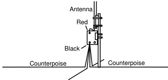
Counterpoise should lie on top of the ground. Do not anchor with a ground rod – it will de-tune the array. The center and far ends of the counterpoise wires may be secured with non-conductive stakes or pins to hold them in place.
