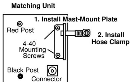
Once the antenna is set up and operating, the network cover may be re-installed without screws to allow for quicker access to the loading coil. The matching unit is generally mounted on the antenna's support pole a foot or so below the antenna base plug.
