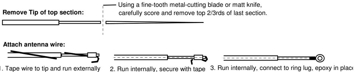
**Procedure for Extending the Antenna Pole:** During set up, the fiberglass pole must be extended to its full length on the ground before being raised into the vertical plane. Also, each section must be pulled out in sequence -- from the smallest to the largest in diameter. If one or more small-diameter sections accidentally slip down behind larger sections during extension, you'll need to remove the base plug and re-nest them so they “telescope” correctly. To extend:
