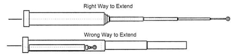
As you extract each section, antenna wire will feed in through the base plug. Make sure nothing blocks the feed. When all sections are extended, about two feet of wire should remain. This pigtail will be connected to the red post on the loading coil box once the antenna is in position. Before raising the antenna, check each section to ensure it is locked securely. If any section fails to lock by twisting, install a couple turns of tape around the joint to temporarily secure it.
