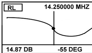
**Phase Angle (Deg):** When a test signal (incident wave) is transmitted to the load under test, the returning signal (reflected wave) will rarely return in phase. This screen plots the phase angle and amplitude ratio between the incident and reflected wave.
