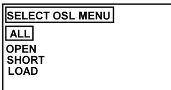
The program will provide you with step-by-step prompts for executing the entire *Open/Short/Load* cal procedure:
