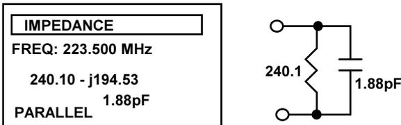
**Screen 5, S11 Scattering Parameters:** Displays Rectangular and Polar S11 representations of the load.
