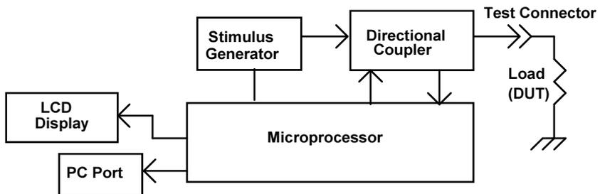
As shown in the diagram above, the analyzer's *DDS RF-Stimulus Generator* (or VFO) generates a test signal that routes through the directional coupler to the load under test. If a mismatch (impedance discontinuity) exists, a portion of that generated signal is reflected back to the load.
