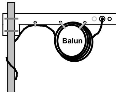
Lower HF Range: Coil 16-18 feet of cable
