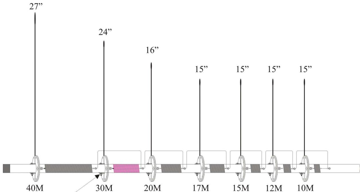
You may loosen the radial ring mounts to make it easier to align the ring holes when inserting the rods. Tighten them back when all four rods are in.
