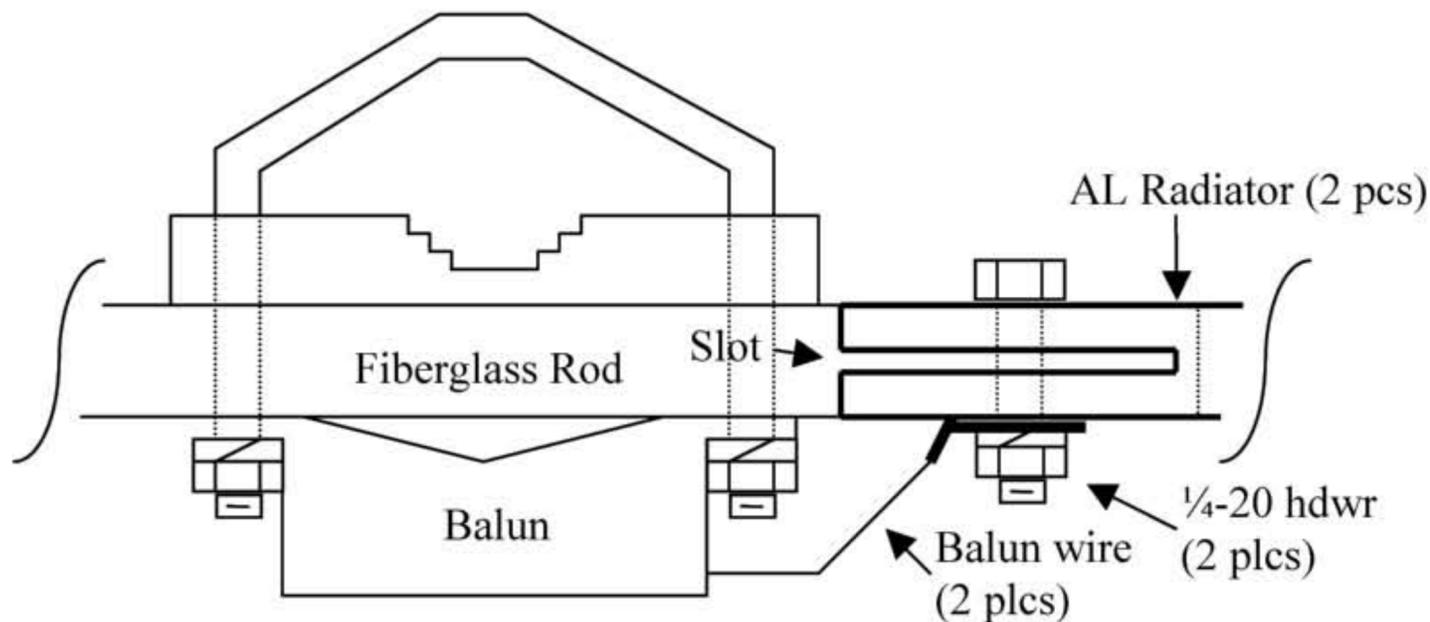
**Figure 3: Radiator Tube Assembly – Top View**
