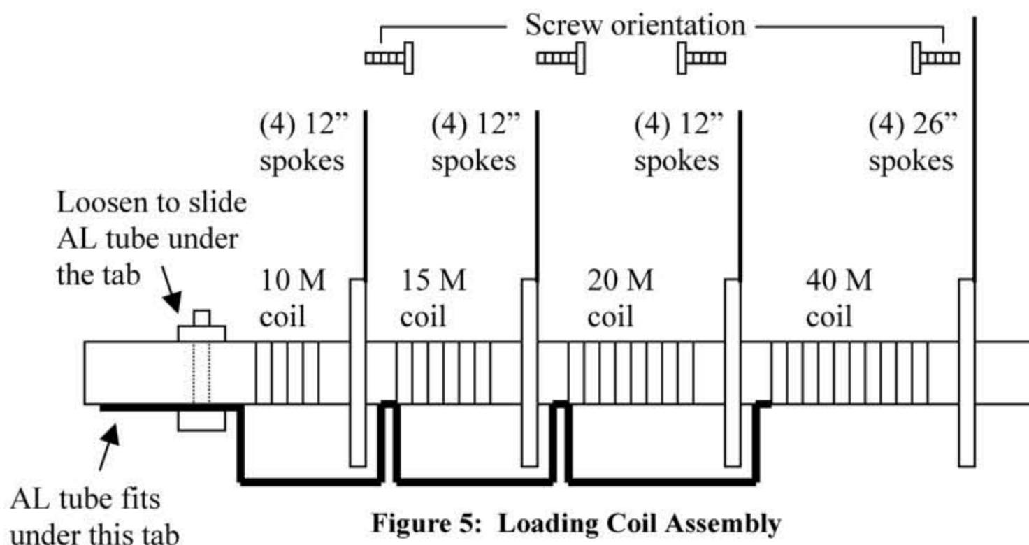
Figure 5: Loading Coil Assembly
