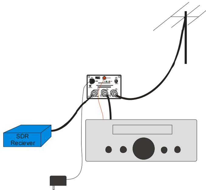
1. Connect the transceiver to the XCVR connector.
