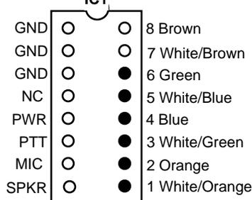
In order for the wiring configurations shown in this manual to work correctly, follow this color code when installing your connector.
