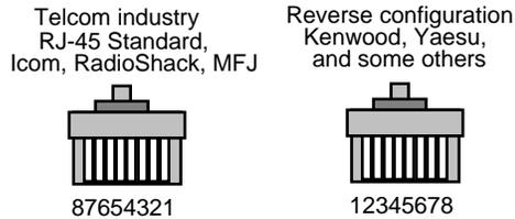
All jumper settings shown in this manual have been corrected to compensate for the reversed pin order used by those manufacturers.
