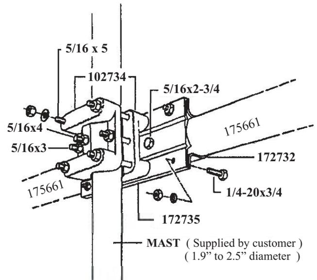
**Note:** If you use a galvanized 1-1/2 schedule 40 or 80 pipe as a mast, it has an O.D. of 1.9". You will need to put two split lockwashers under the 5/16 nuts on the four long bolts.
