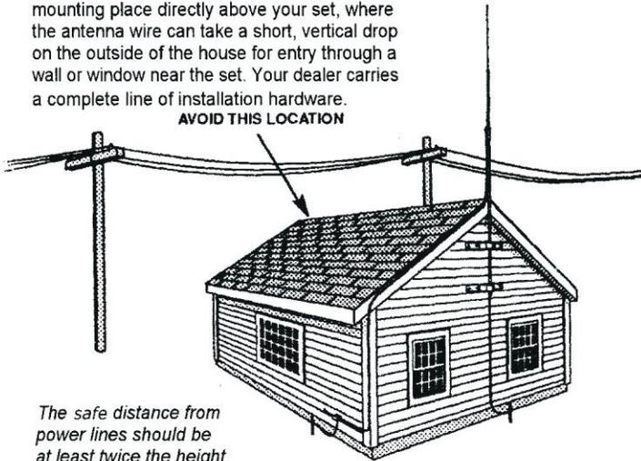
*The safe distance from power lines should be at least twice the height of the antenna and mast combined.*
