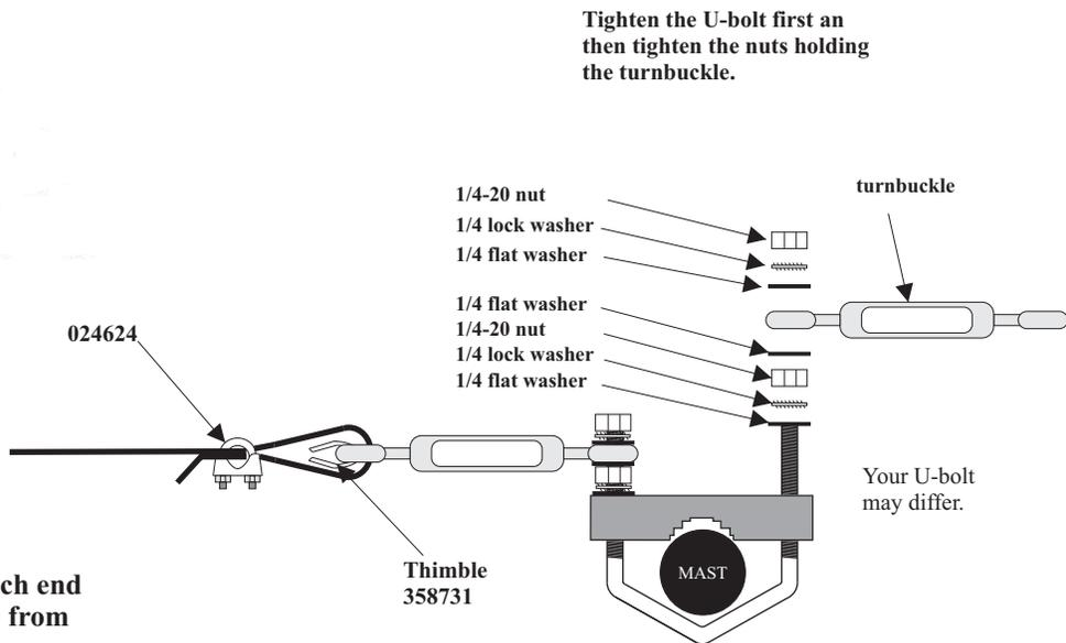
Place support clamp about 3 feet above the boom clamp. Use left over rope to prevent turnbuckle from rotating after installation by routing it through the eyelets. Pull the rope tight and tie it off. You may use cable ties or other means of securing the turnbuckle if you wish.
