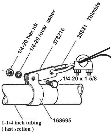
Install the tube clamp at the last joint on each end of the antenna. This will prevent the clamp from slipping.
