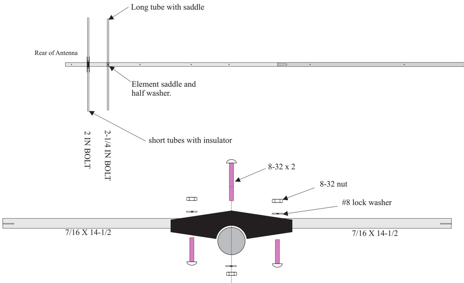
Mount the insulator on the Boom at the second hole from the rear of the antenna using the  $8-32 \times 2$  inch bolt. Attach the two short  $7/16$  tubes to the insulator using the  $8-32 \times 1$  inch bolt thru the holes in the ends of the tubes. Go ahead and tighten the nuts but do not crush the tubes.
