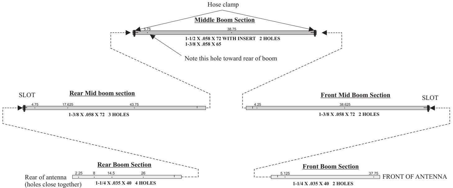
Insert each tube 3 inches into the next using the marks you made. Try your best to align the holes in each tube. Tighten the hose clamps just enough so that the tubes do not move. Final alignment of the tubes will likely be needed later. Now would be a good time to support the boom on a couple of saw horses or something similar.
