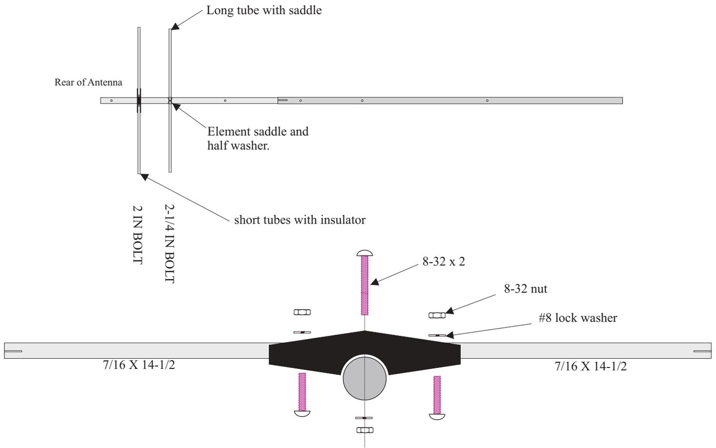
Mount the insulator on the Boom at the second hole from the rear of the antenna using the 8-32 x 2 inch bolt. Attach the two short 7/16 tubes to the insulator using the 8-32 x 1 inch bolt thru the holes in the ends of the tubes. Go ahead and tighten the nuts but do not crush the tubes.
