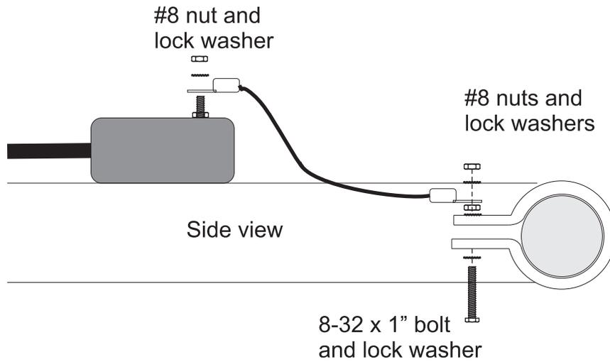
Use cable ties or electrical tape to secure the coax and balun to the boom of the antenna
