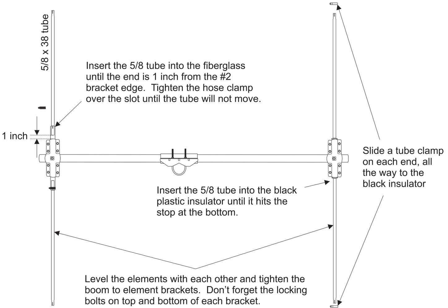
Assemble the antenna as shown in the diagram on the next page. Do not over tighten the hose clamps as it will damage the worm gear.
