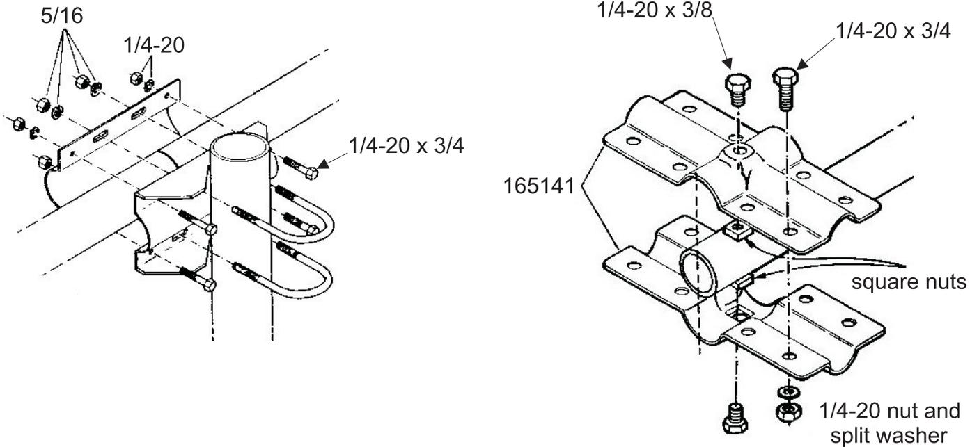
Loosely assemble the #2 boom to element brackets for each end of the antenna. Slide them over each end of the boom. Insert the fiberglass insulators into the brackets with the slot outward. Insert the black plastic insulators into the other end. It doesn't matter which end you choose for each type insulator. Push the insulators all the way in and snug the bolts so that they will not fall out.
