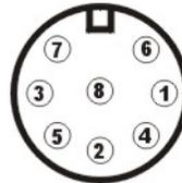
**NOTE: Ground is connected to the outer shell of the 8-pin din plug. Failure to connect ground to the outer shell will result in the relay box not operating correctly.**
