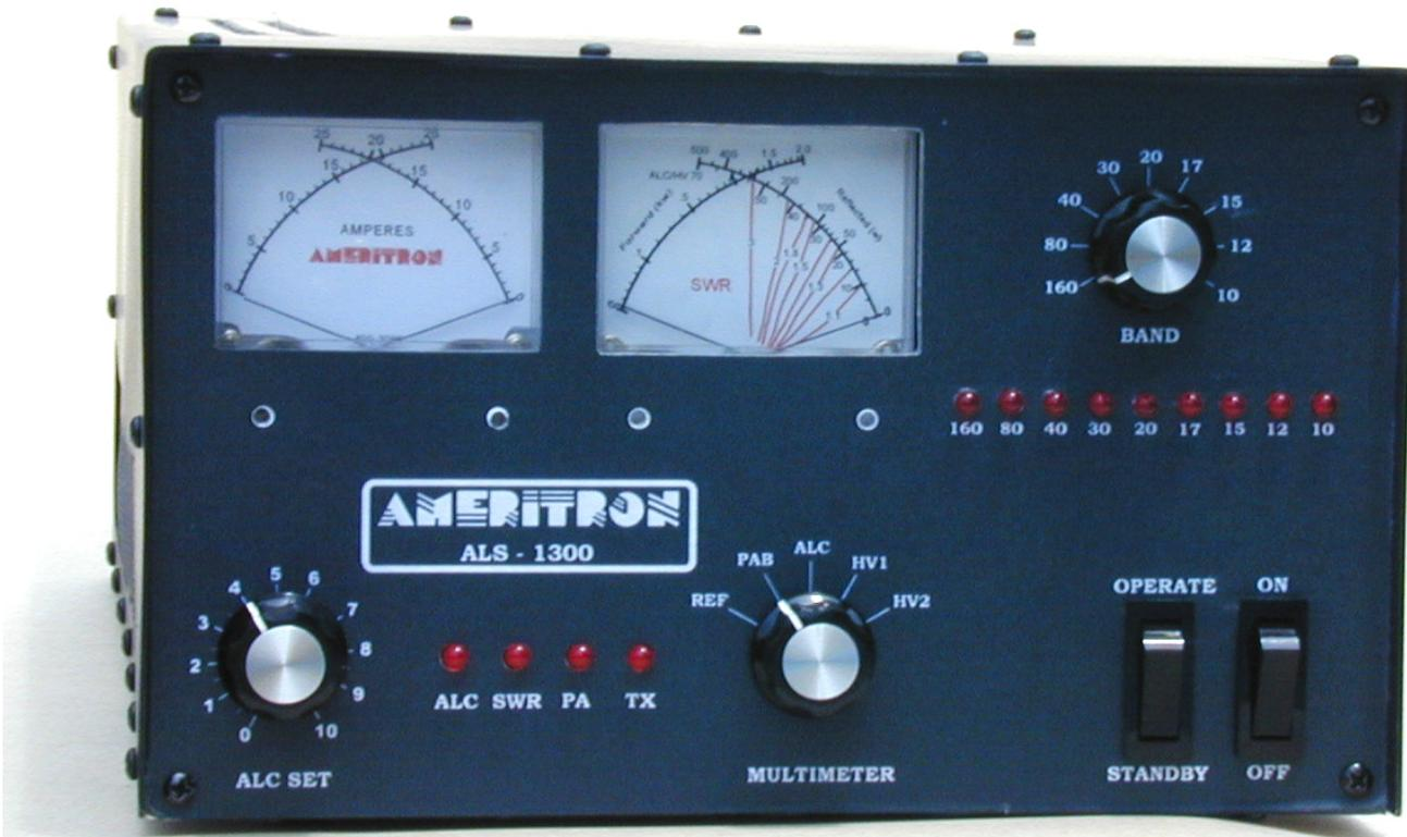
The Ameritron ALS-1300 is a 160 through 15-meter 1200-watt output solid-state amplifier. An optional user-installed MOD-10MK filter assembly extends operation to 12- and 10-meters. The ALS-1300 uses eight 50-volt conservatively rated linear RF MOSFETS. These 50-volt linear FET's produce an exceptionally clean signal compared to other solid-state amplifiers. Fan speed is regulated by temperature sensors assuring conservative cooling with minimum noise.
